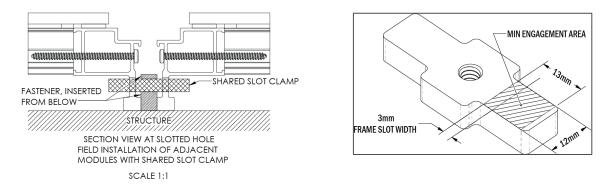
Figure 7: Shared SpeedSlot Clamp Detail
