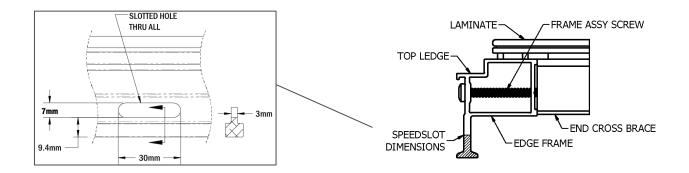
Figure 5. SpeedSlot Dimensions
