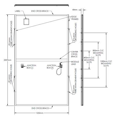
Figure 3: Series 6 Module Mechanical Drawing
