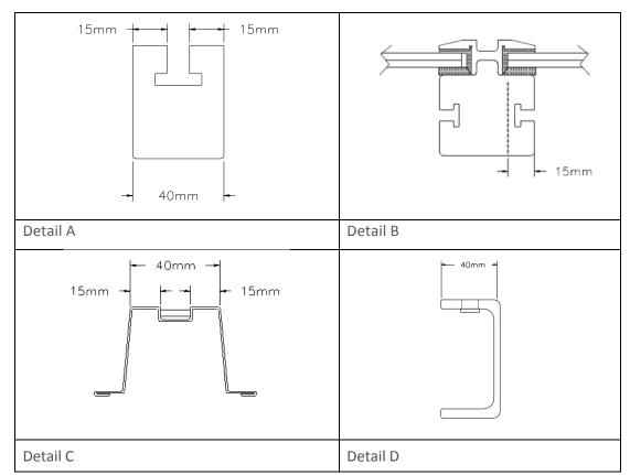
Figure 6. Module rail sample profiles and critical rail dimensions
