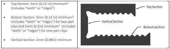
Figure 7. Clip Insulator Minimum Dimensions
