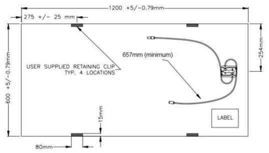
Figure 2. Recommended Location of Retaining Clips (back side)
