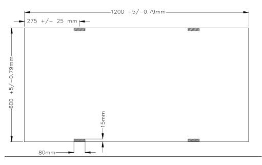
Figure 1. Recommended location of retaining clips (front side)
