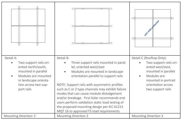
Figure 4. Support Rails and Module Orientations
